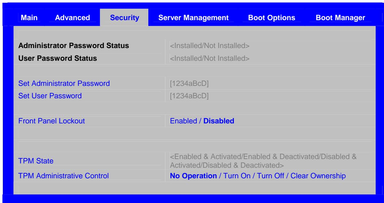
Figure 11. Setup Utility – TPM Configuration Screen
