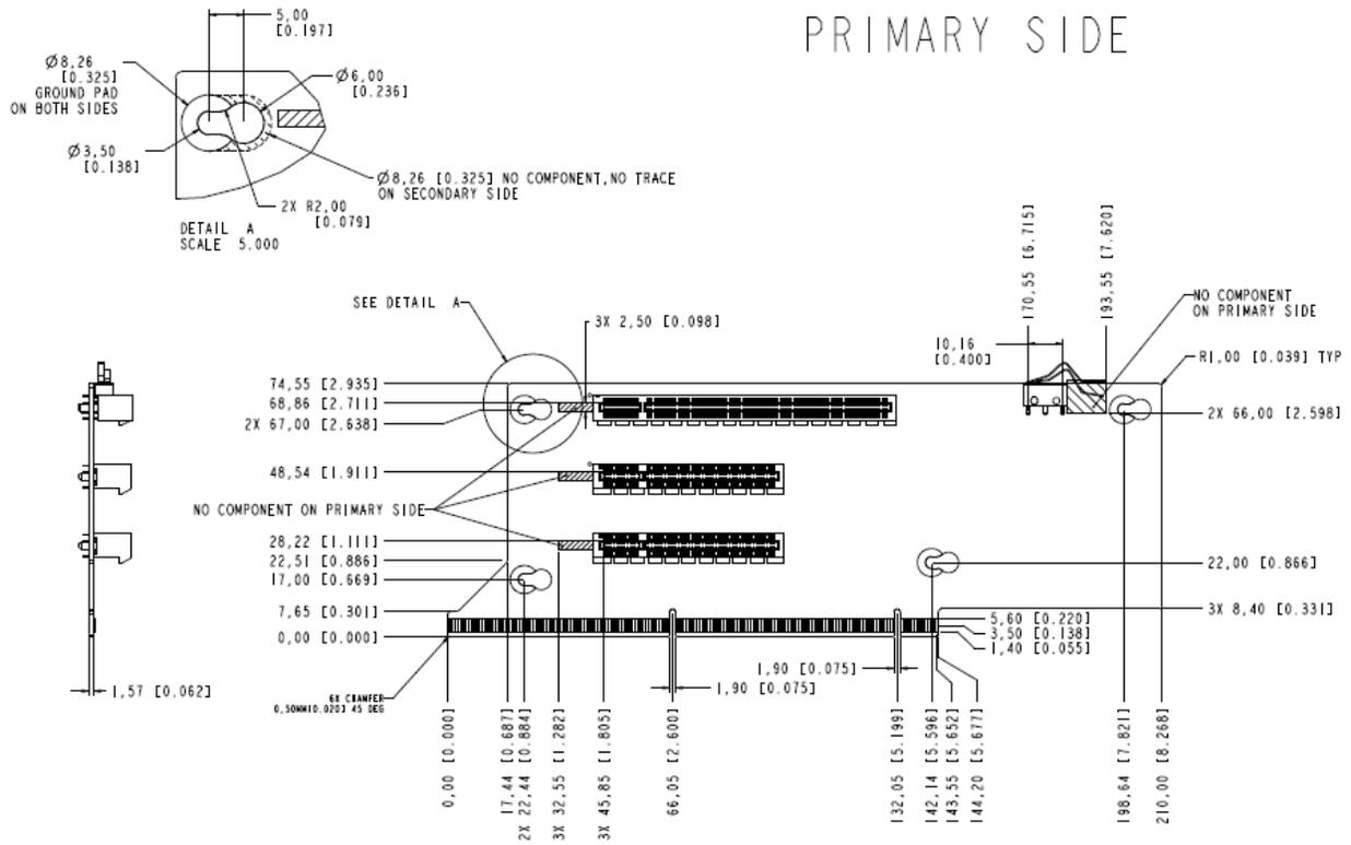
Figure 46. 2U PCI Express\* Passive Riser – Primary Side
