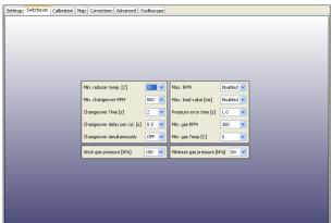
a) set desired parameters for system change over To Gas and To Petrol.
