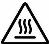
Temperature Hazard Caution or Warning
