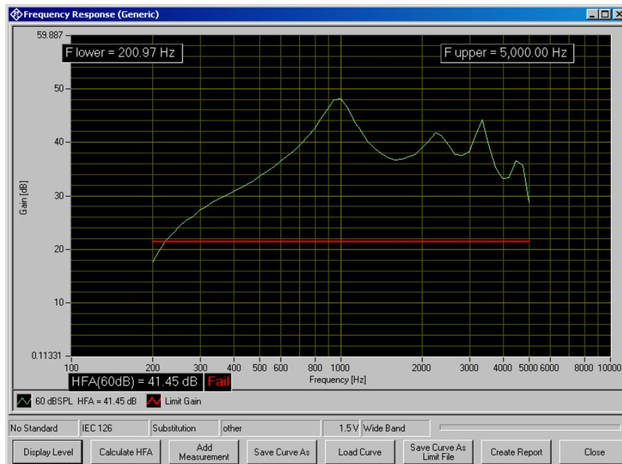
Fig. 31 Display window of frequency response measurement
