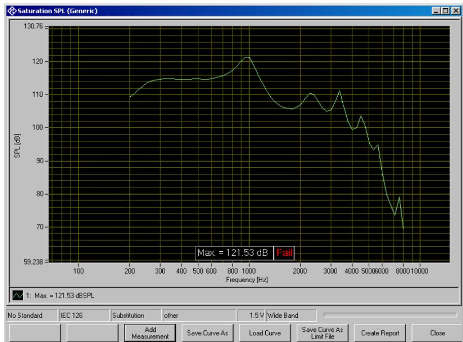
Fig. 35 Display window of saturation sound pressure level measurement
