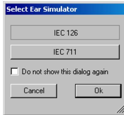
Fig. 5 Query window for selection of ear simulator
