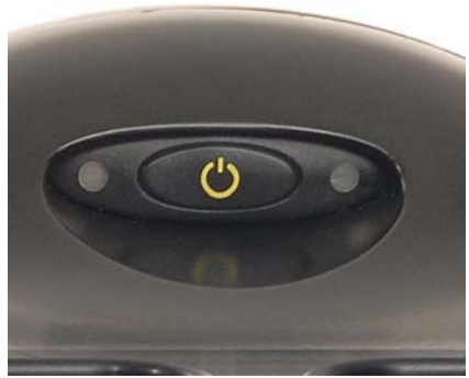
Fig. 08. Engage switch. LED-indicators to the left and right.
