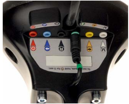
Fig. 02. The connection panel located on the Occipital Pad. Showing input ports for 3.5 mm jack connectors.
