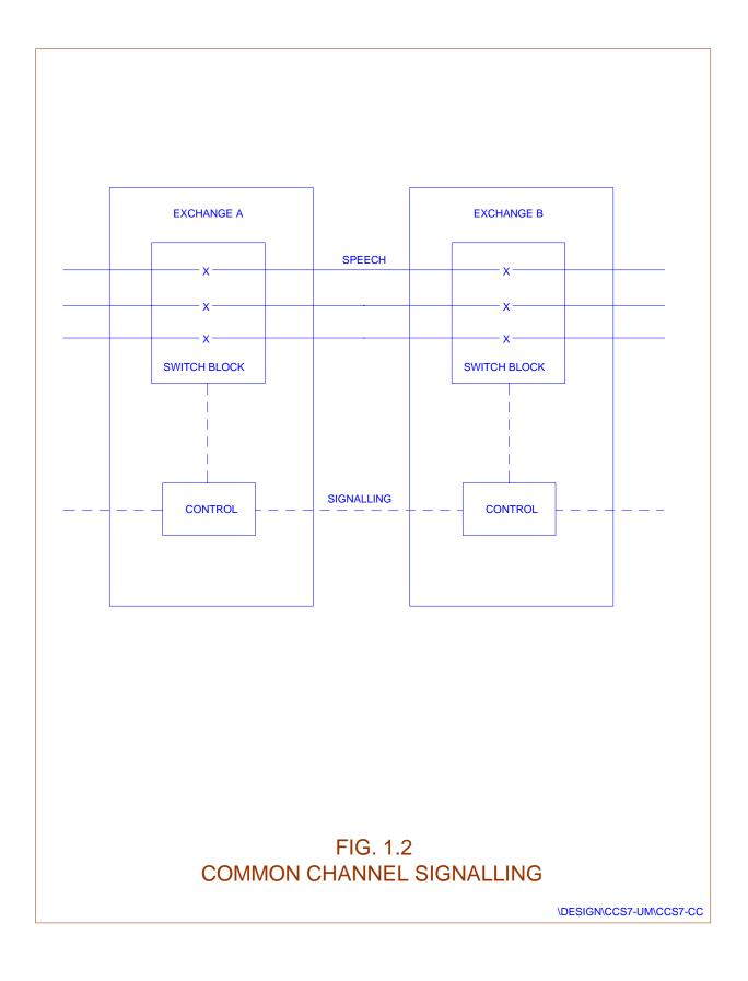
One result of the evolutionary process of exchanges described above is to change the relationship between signalling and call control. In the early exchange systems, exchanges could communicate, but in a limited and inflexible manner, thus limiting the flexibility of call control. In a CCS environment, the objective is to allow uninhibited communication between exchange control functions, or processors, thus tremendously broadening the scope and flexibility of information transfer.
