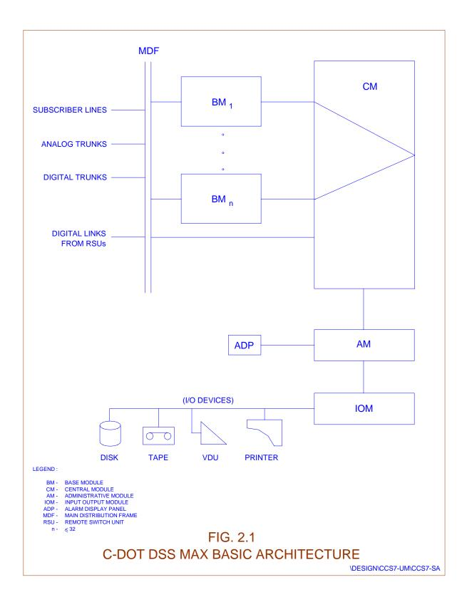
The duplicated Network Synchronisation Controller (NSC) in the CM provides clock and synchronisation to processing complexes in the switch. It has digital phase locked (PLL) circuitry for locking to the network reference clock. In free-run made, it supplies its highly accurate (level 2) clock to the switch.
