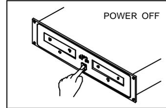
Switch off the power after the disc holder has been closed with the OPEN/CLOSE button.
