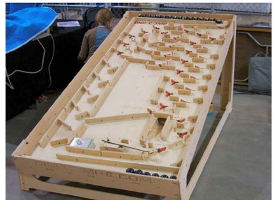
Giant Digi-Comp II by Evil Mad Scientist Laboratories is an oversized recreation of the Digi-Comp II, a mechanical educational computer from the 1960s that used marbles to perform simple calculations. Giant Digi-Comp II was on display at Maker Faire Bay Area 2011. Kits will be available for purchase at Evil Mad Science this summer. http://laughingsquid.com/giant-digi-comp-ii-recreates-mechanical-computer-from-1960s/
