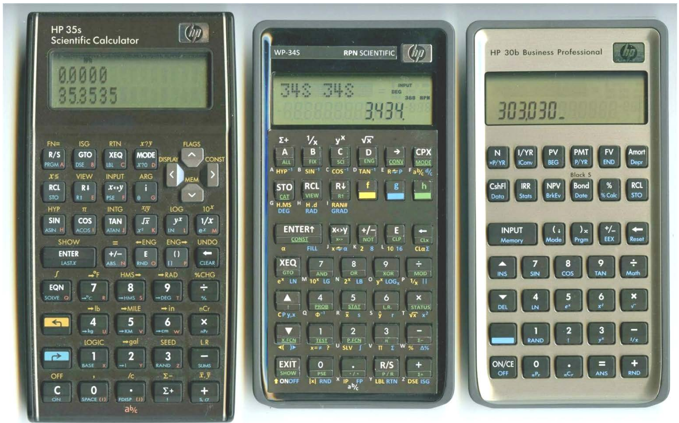
Figure 1. (Left to right :) HP 35s scientific; WP-34S scientific repurposed from an HP 20b; HP 30b business calculator. The 34S utilizes one of Eric Rechlin’s professionally-made keyboard overlays and individual key covers.
