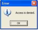
If this dialog box displays COM 1 was either not installed or already in use. Just select the correct port under the port tab and you should be connected to the reader. A check mark next to the port and to open indicates that the port is connected.
