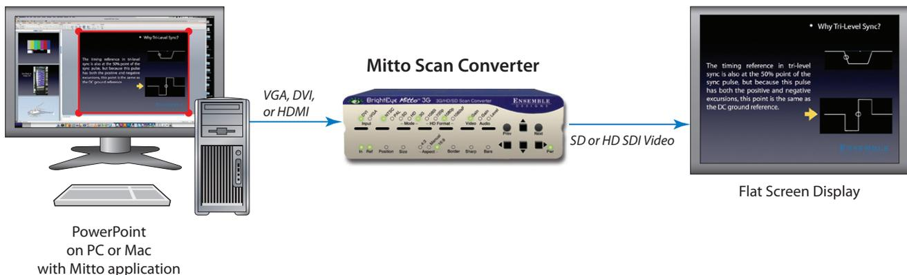
*The above illustrates how you can connect your Mac or PC to the BrightEye Mitto through the VGA, DVI or HDMI port on your computer. Mitto outputs composite, SD or HD video that can be fed into a monitor or production switcher.*
