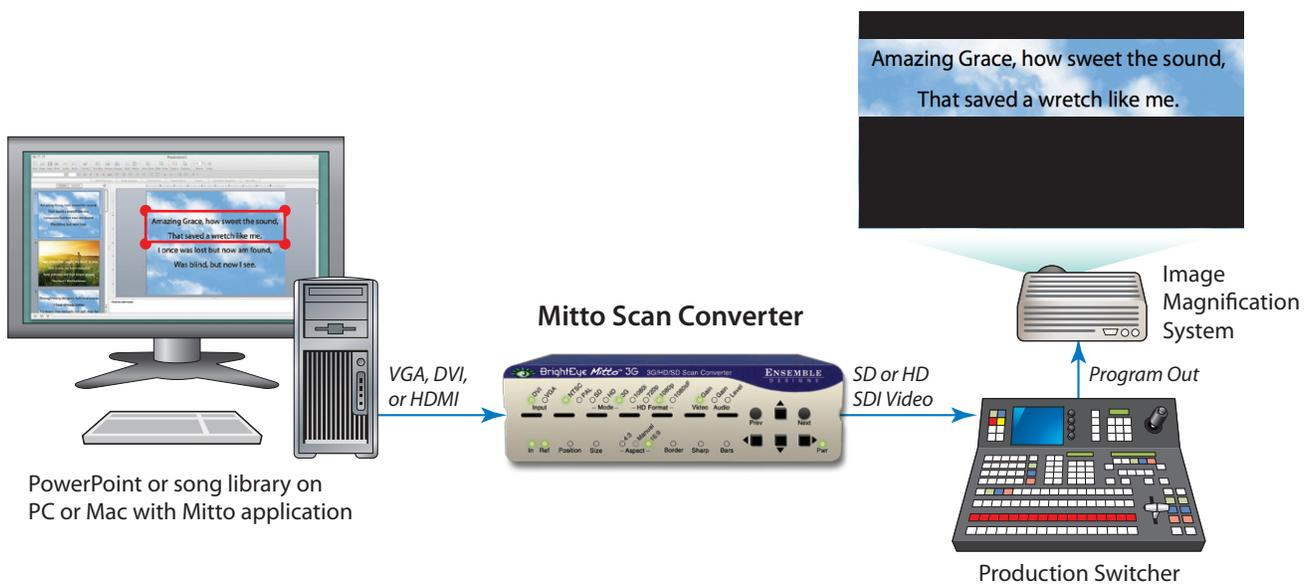
*The above illustrates how you can select just a portion of the song or hymn lyrics for scan conversion. Feed Mitto's SD or HD SDI output to a video switcher or iMAG system.*
