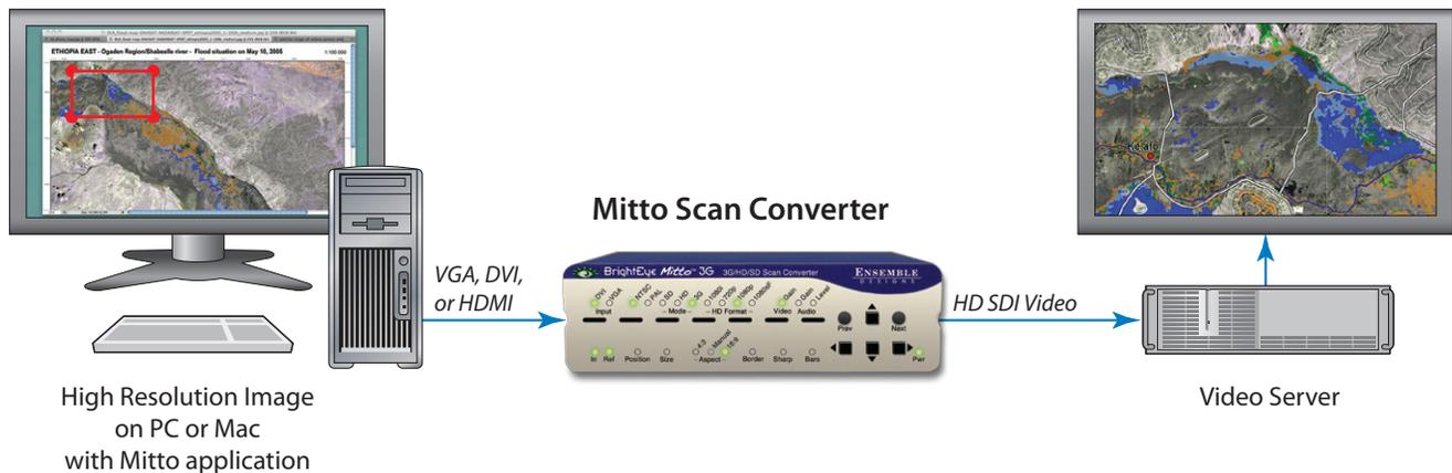
*The above illustrates how you can use BrightEye Mitto to output detailed maps to HD SDI video. Connect your Mac or PC to the BrightEye Mitto through the VGA, DVI or HDMI port on your computer. Mitto outputs full 1080p 3 Gb/s HD video for superior detail.*
