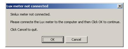
Please connect Simlux meter to the PC and put the Simlux meter in the Calispector testing window. Click OK to continue and Calispector will indicate the estimated time for the calibration.
