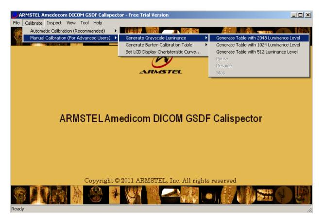
Click Manual Calibration-> Generate Grayscale Luminance-> Generate Table with 2048 Luminance Level, it will indicate the following:
