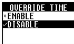
7. Enable or disable the override time. This is the time after a sample will be drawn even if the accumulated flow has not reached the total specified in step 6.
