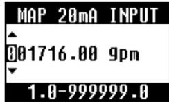
5. Enter the flow rate for the 20mA input.
