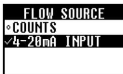
3. Select the units used to specify the flow rate while mapping the 4mA and 20mA inputs.
