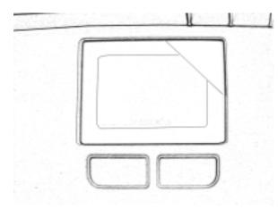
TOUCHPAD surface can be use to move the cursor in the GUI environment by placing and moving your finger. The two buttons located below the touch pad act as same as the mouse left/right button. Or you may wish to tap on the touch pad to indicate a left click.
