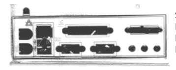
SAX 903/906 : 1x 25pin Parallel Port, 1x 9pin COM Ports, 2 x USB Ports, 1 x Ethernet RJ45.
