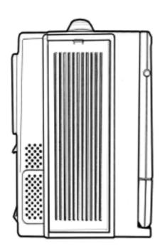
The side panel is located behind the plastic protection cover that can be removed by pushing the clip. Depending on the system board and your add-on cards, you may also have other ports such as Ethernet port, and Audio ports. When in use, side panel can also be stored in a slot located on the back cover
