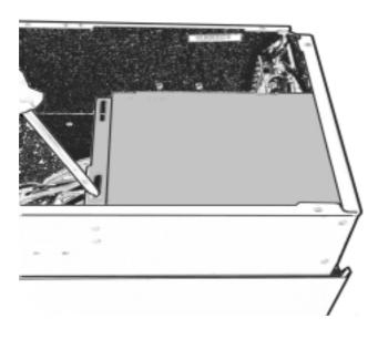
\* Be sure reinsert the hanger before taking off the Power Supply, there are two more screws to screw..
