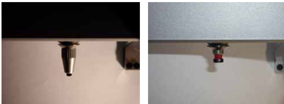
Figure 19 The button extension (left) and removed (right)
