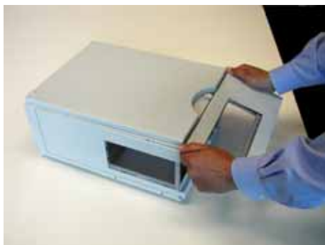
Figure 1 Removing the front door of the Autosampler
