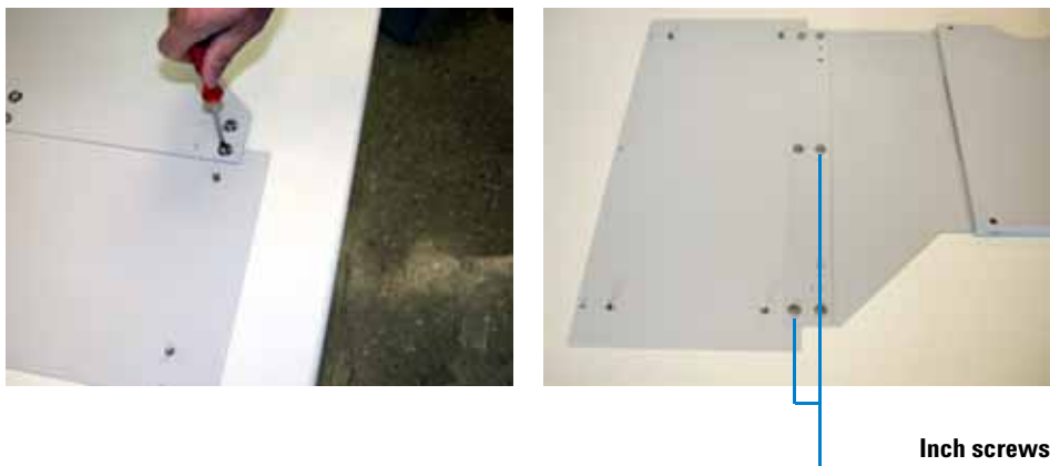
Figure 12 Assembling the sheet metal parts
