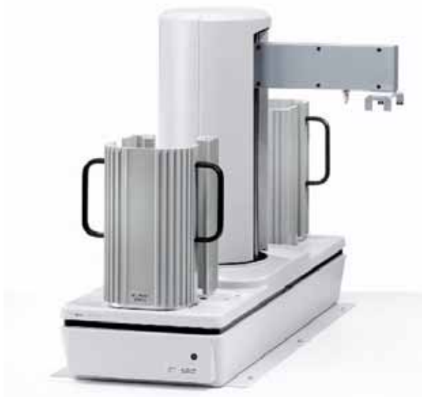
Figure 21 Input and output racks on the Well-plate Handler
