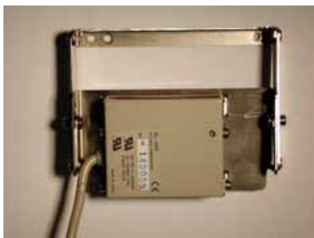
Figure 27 Barcode reader mounting position for landscape position
