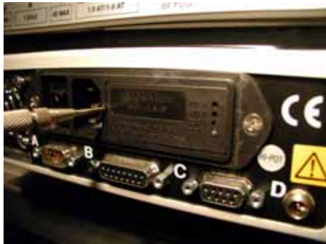
Figure 13 Prying open the cover/fuse-block assembly
