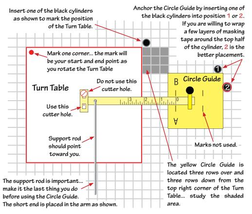
To Check Your Setup: Set the scale to zero... insert a pencil into the cutter hole and spin the turn table. If your setup is correct you will draw a dot or small circle on the turn table... a larger circle means your setup is not correct. The center of the dot or circle is the center of the turn table.
