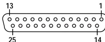
**Illustration 2-7 Remote I/O connector (back panel view)**
