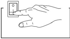
9. Place the Local/Remote switch (see Illustration 3–2) in the Remote position and, using an external remote control unit connected to the Remote I/O connector or the on-board remote Raise/Lower buttons, adjust the PA2000 to the maximum power set by the Local Power Adjust. (This prevents adjusting to higher than permitted power levels.)
