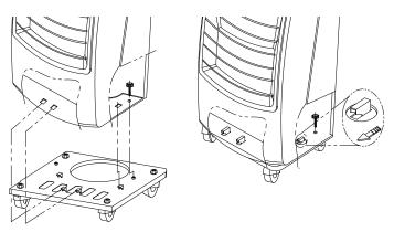
Figure 2. Removing/Replacing Bottom Plate
