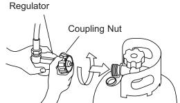
Figure 3. Connecting Hose/Regulator to LP cylinder
