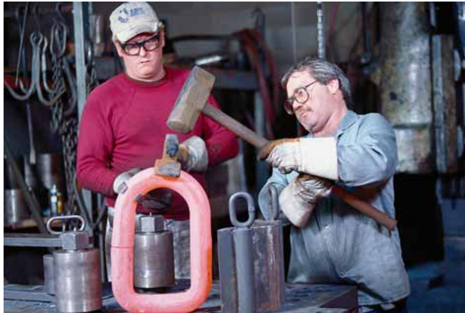
Forming Red Hot D Link from 2" Material for Magnet Chain Master Link.
