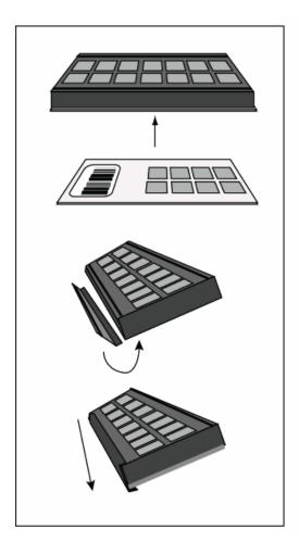
Carefully place slide at bottom of the chamber as shown. The slide will adhere somewhat to the bottom. Warning: the slide is fragile, so do not apply more than gentle force to the apparatus.
