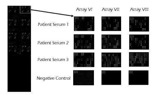
Note the 6 strong signals of the Positive Control spots in the upper-left corner. These spots are useful for proper orientation of the array image.
