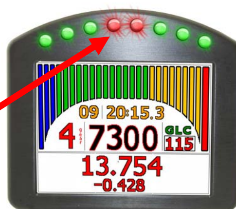
Figure 18 – Micro Pod With Shift Lights
