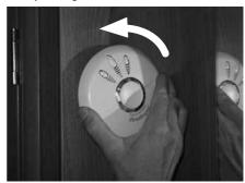
Remove the existing battery and replace with a new battery. From the list on this page, making sure that the positive and negative connections are in the correct position. If unsure see the alarm user manual.
