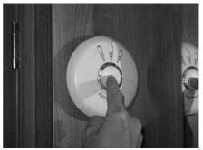
The unit will emit a loud (85dB at 3 meters) alarm for around 5 seconds and stop automatically.
