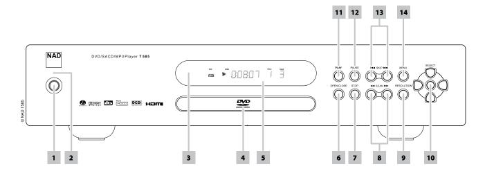
1 **POWER BUTTON:** Press this button to switch ON the T 585. The LED indicator will turn from amber to green and illuminate the VFD. Pressing the power button again turns the unit back to standby mode.
