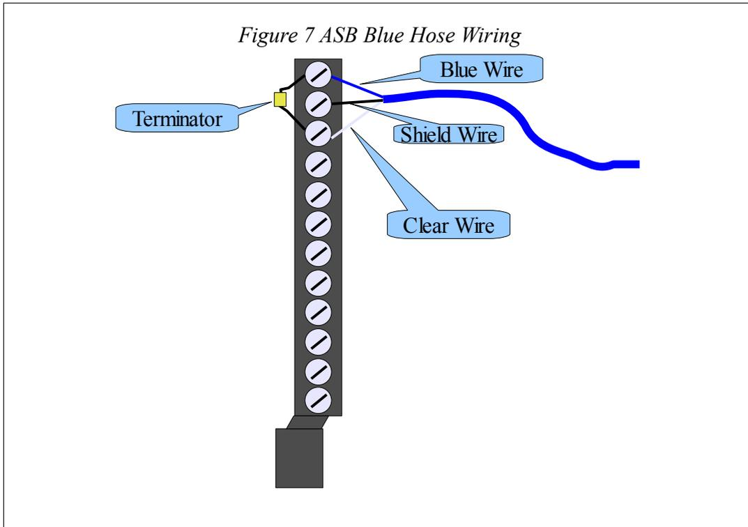
The wiring of the ASB card simply connects the “Blue Hose” cable to the proper screw terminals. Also notice that since this is the last node on the network the 82ohm terminator is also installed across the clear and blue wires.
