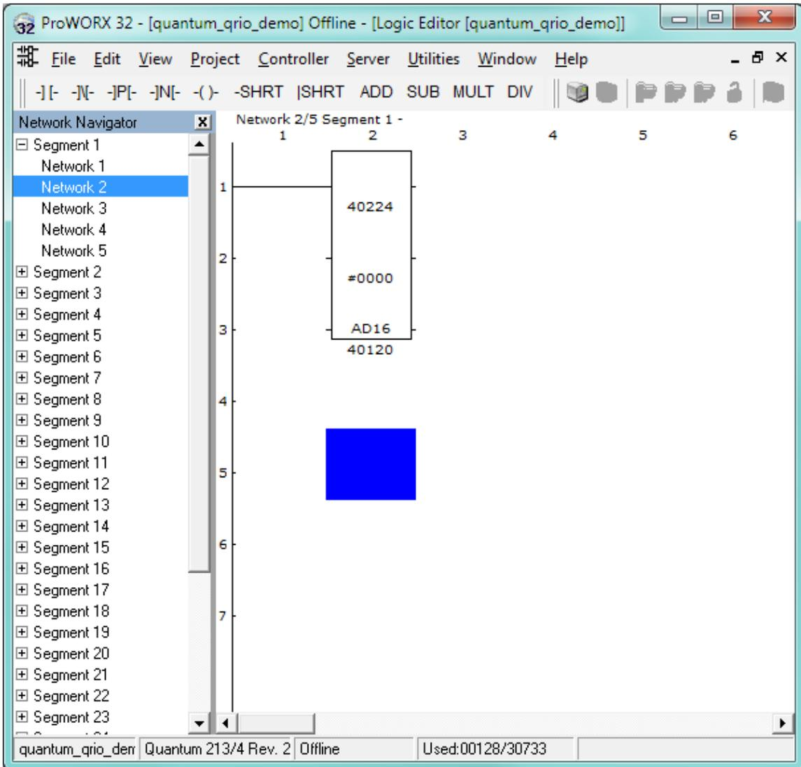
Figure 12: Copy Analog IN 1 Value to Analog OUT 1
