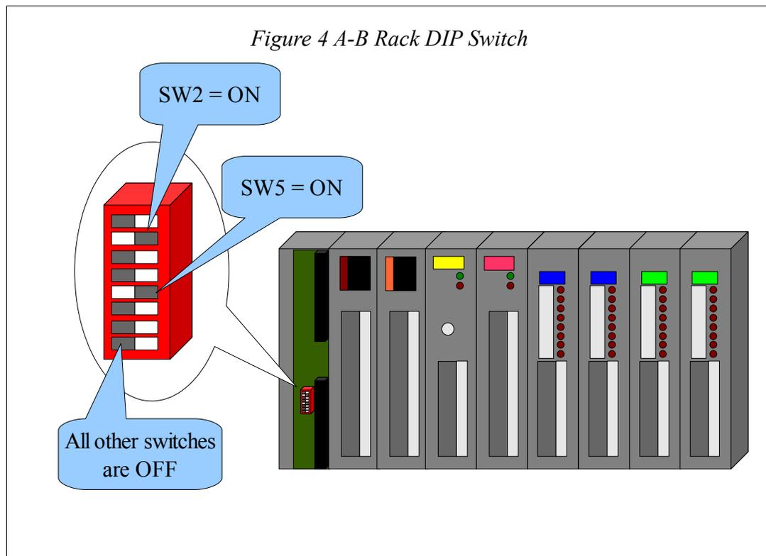
The implication of 1-slot addressing is that every slot in the rack has 16 input bits and 16 output bits assigned. This wastes a lot of bits, but it is the only way to make it work. Sixteen bit input only cards use all 16 input but waste the 16 output bits. Output
