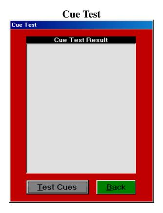
In order to do 'Cue Test', a script must be loaded into memory. Go to either 'Sync Show', 'Timed Show' or 'Manual Show' and load the desired script. Then 'Back' out and press 'Cue Test'. Pressing 'Test Cues' will check the chosen script with the attached cues. For every cue specified in the script, 'Test Cues' will test for continuity. It will report back on the screen the status of all cues.
