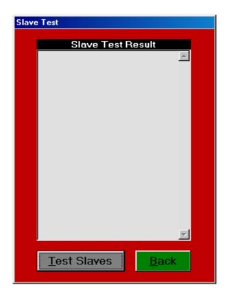
In order to do 'Slave Test', a script must be loaded into memory. Go to either 'Sync Show', 'Timed Show' or 'Manual Show' and load the desired script. Then 'Back' out and press 'Slave Test'. It will check to see if those modules are connected and communicating with the computer. It will then report back on the screen all the Slaves connected and their status.
