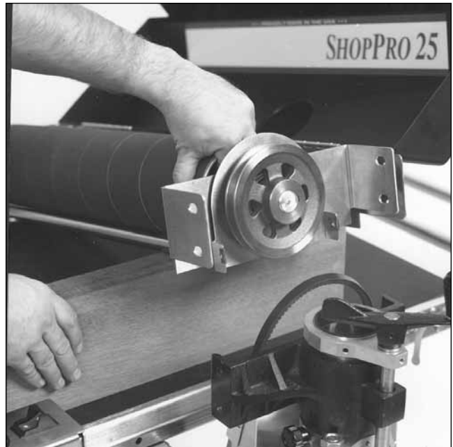
Fig. 32. Supporting drums with 2x6 on edge.
