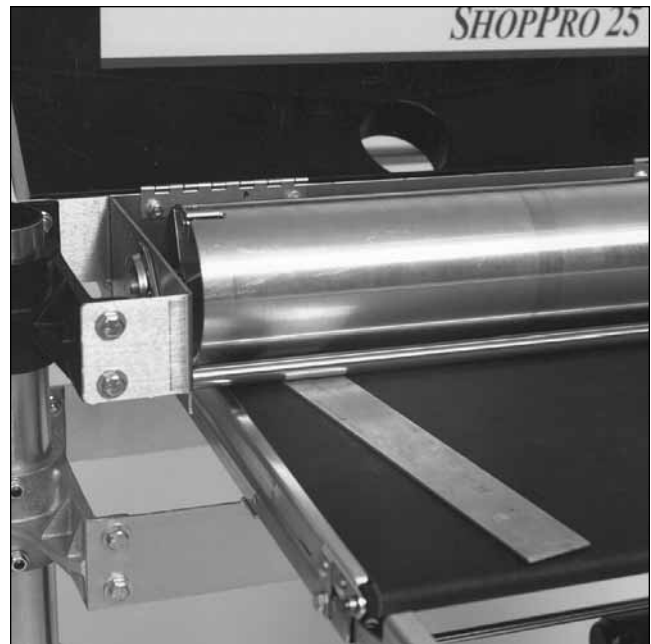
Fig. 26. Using thickness gauge during alignment.
