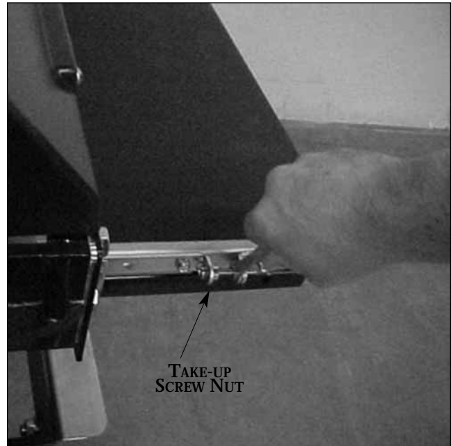
Fig. 10. Adjusting conveyor belt tracking.
