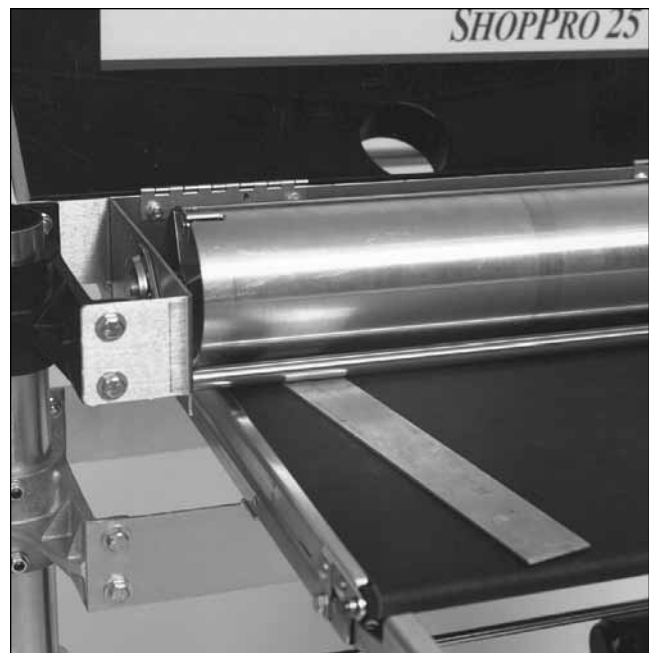
Fig. 7. Checking drum alignment (outboard side).
