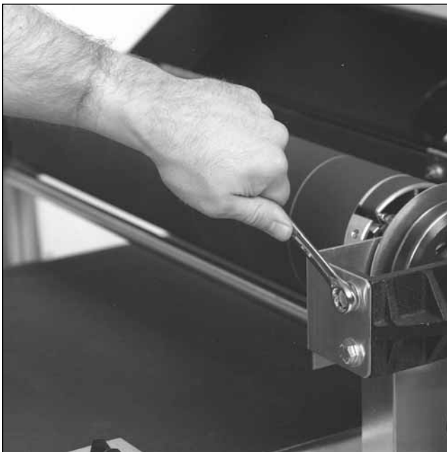
Fig. 30. Removing bolts from inboard drum support casting.
