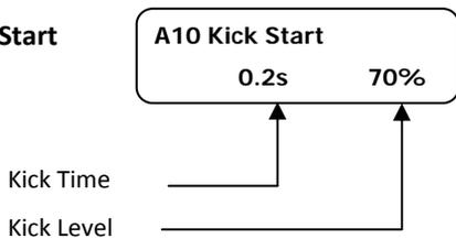
Set to provide a kick during starting. This provides an adjustable torque boost to the motor when a start is initiated. This will also result in a higher start current during the kick duration.
