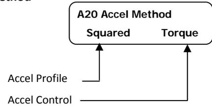
The acceleration method allows adjustment of the acceleration profile and acceleration control. This provides advanced control of the motor during the ramp time to better match the type of load or application. See Appendix A on Page 42 for more details.
