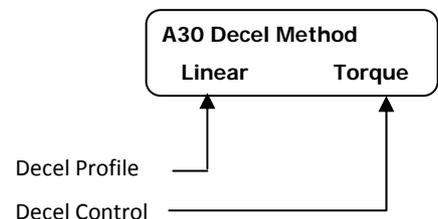
The deceleration method allows adjustment of the deceleration profile and acceleration control of the Soft Starter. This provides advanced control of the motor during the ramp down time to better match the type of load or application. This is especially useful in resolving water hammer related problems.
