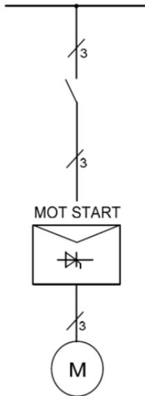
**3Wire / 6wire:** The standard connection of an electronic soft starter is 3 wire. An alternative connection is 6 wire or inside delta connection. This is commonly used when replacing a star/delta type motor starter.
