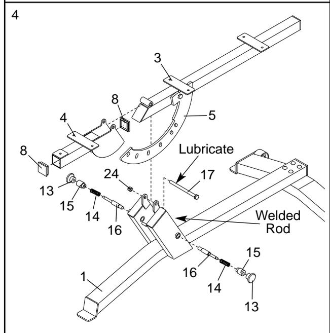
Engage the lower Adjustment Pin (16) into the Adjustment Arm (5). Engage the upper Adjustment Pin into the Seat Frame (4). **Make sure the Pin is in the center of the hole in the Adjustment Arm. Tighten the two M10 Nylon Locknuts (not shown) used in step 3.**
