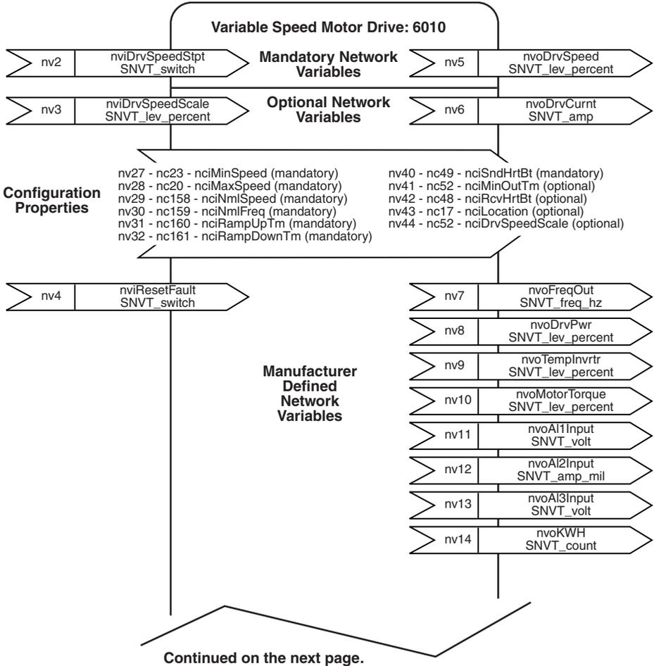
**Figure 6: Variables and Configuration Properties in Drive Object**
