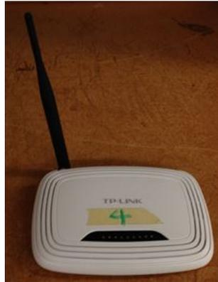
Fig. 4.2: TL-WR740N WiFi router used in the indoor positioning module
