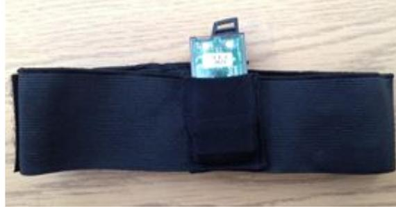
**Fig. 2.7:** SensorTag customized Velcro strap
