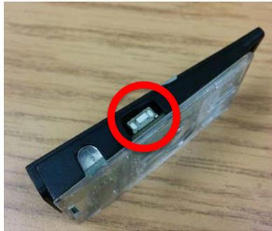
Fig. C.6: SensorTag ON/OFF switch encircled in red
