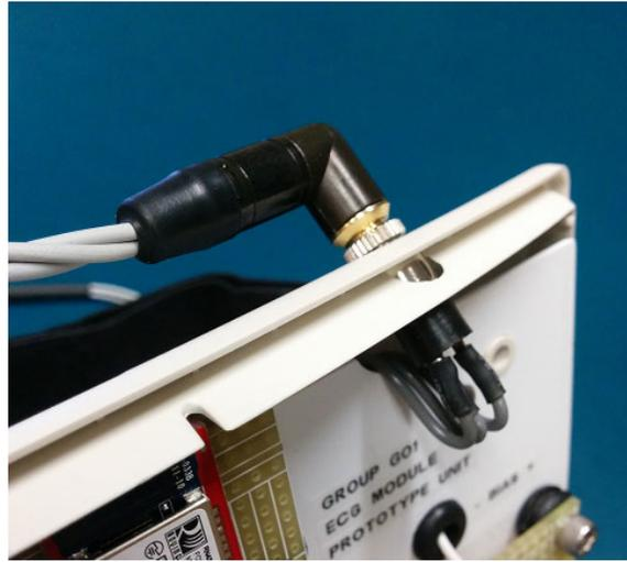
**Fig. 3.8:** 3.5 mm stereo plug and jack electrode lead connection
