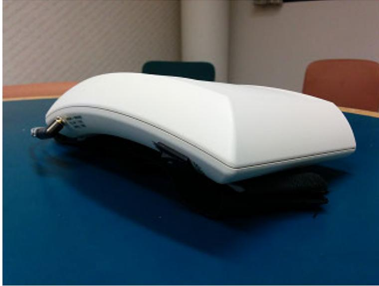
**Fig. 3.10:** ECG module enclosure with lid affixed
