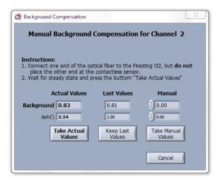
Here the background fluorescence of the connected *Optical Fiber* can be compensated. For this it is *important* that
