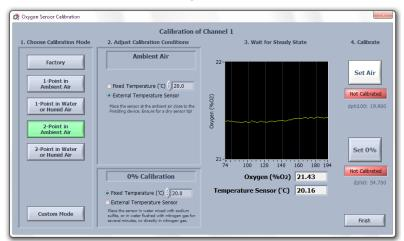
For the air calibration value (**Ambient Air**), place the oxygen sensor and the external temperature sensor (if used) **close to the air holes** at the backside of the *FireStingO2*.
