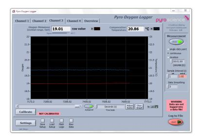
The four panels **Channel 1-4** correspond to the channels 1-4 of the fiber-optic oxygen sensors connected to the *FireStingO2*. For the 1- or 2-channel version of the *FireStingO2*, only the respective panels will be visible.
