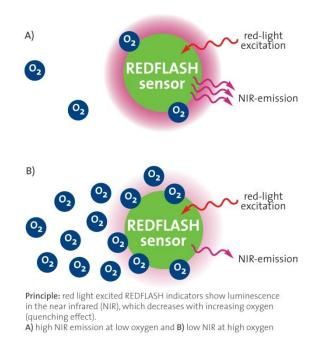
The **REDFLASH technology** impresses by its high precision, high reliability, low power consumption, low cross-sensitivity, and fast response times. The red light excitation significantly reduces interferences caused by autofluorescence and reduces stress in biological systems. The **REDFLASH indicators** show much higher
