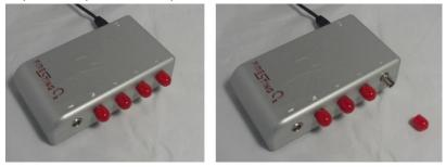
Then insert the male fiber plug (**M**) of the sensor cable into the ST-receptacle (female fiber connector) of the *FireStingO2* and turn the bayonet coupling gently clockwise until the plug is locked firmly.
