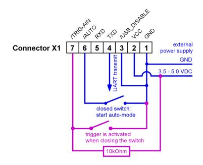
This configuration is almost identical to the preceding case, only the power supply is now given at pins 1 and 2. The USB connector of the *FireStingO2* is left unconnected. Note the additional connection between pin 1 and 3 powering down the internal USB interface of the *FireStingO2*.
