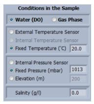
If **External Temperature Sensor** or **Internal Temperature Sensor** (in a Gas Phase) is selected, automatic temperature compensation
