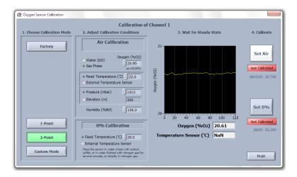
The air calibration standard and the calibration conditions need to be defined and entered as described for the **1-Point** calibration (see chapter 7.2.2).
