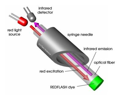
The measuring principle is based on a sinusoidally modulated red excitation light. This results in a phase-shifted sinusoidally modulated emission in the NIR. The *FireStingO2* measures this phase shift (termed "dphi" in the software). The phase shift is then converted into oxygen units based on the Stern-Vollmer-Theory.
