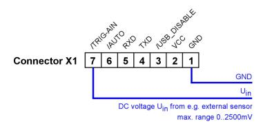
For reading in voltage signals between o and 2.5 VDC of e.g. an external sensor, simply connect the voltage to pin 1 and pin 7. Ensure a correct polarity. And ensure that the voltage does not exceed 2.5 VDC. Voltages above 3.3 VDC might damage the device.
