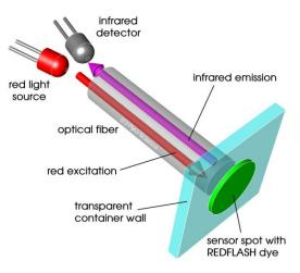
The sensor spots allow oxygen measurements in closed vessels in combination with the *FireStingO2* equipped with *Optical Fibers* (e.g. item no. *SPFIB* or *SPFIB-CL2*). The sensor spots have standard diameters of 5 mm (item no. *OXSP5*) and can be optionally obtained with an optical isolation (black coating) on the sensing surface (e.g. item no. *OXSP5OI, OXSG8OI*). Optical
