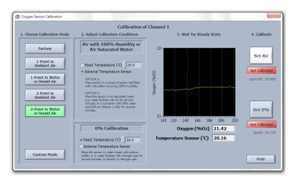
Note, that this calibration mode will automatically read the atmospheric pressure from the internal pressure sensor in the *FireStingO2*. The calibration standards must be therefore exposed to the same atmospheric pressure (which is given in typical applications<sup>3</sup>).
