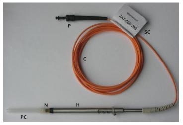
The oxygen-sensitive *REDFLASH indicator* is immobilized at the tip of the sensor, which can be retractable (R) or fixed (F) in the housing.  $\mathbf{R}$
