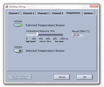
After activation of a temperature sensor in the oxygen channels (see 6.2.3), the measured temperature by the external or internal temperature sensor is displayed in the panel(s) of the corresponding oxygen sensors with activated automatic temperature compensation (right-hand side y-axis). It is also displayed in the **Overview** panel (see chapter o) of the main window and saved into the data file.
