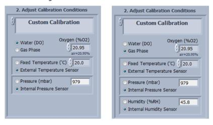
The oxygen level in the calibration standard can be freely chosen in **Oxygen (%O2)**. If the air calibration standard is based on ambient air or air saturated water, then this value should be kept at 20.95%O2, representing the standard oxygen volume fraction in ambient air. However, other values can be adjusted if custom calibration gases are used, of e.g. 5%O2, which might be useful when using trace oxygen sensors.
