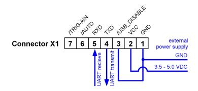
This configuration is used if the *FireStingO2* should be controlled completely via the UART interface by external custom electronic equipment (OEM applications). Note the additional connection between pin 1 and 3 powering down the internal USB interface of the *FireStingO2*. Otherwise unintended data communication via a potentially still connected PC might disrupt the UART communication. More information is available on request.
