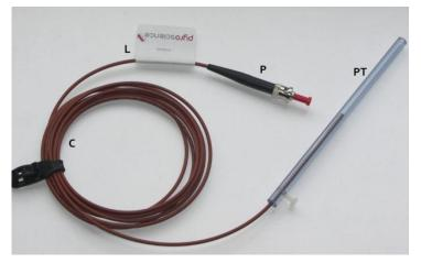
The protective plastic tube (**PT**) covering the bare fiber has to be removed carefully before using the sensor. For this, fix the plastic tube in a stable laboratory stand, loosen the clamping screw and carefully pull out the bare fiber sensor.
