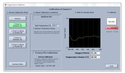
Wait now until the sensor reading is stable by observing the graph and the numerical display of the oxygen sensor reading. If **External Temperature Sensor** was selected, ensure also stable temperature readings indicated at **Temperature Sensor** (°C). Note that the button **Set Air** will be highlighted as soon as the oxygen readings are within the expected range for the connected sensor type.
