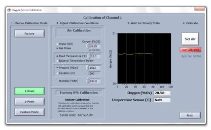
The oxygen level in the calibration standard can be freely chosen in **Oxygen (%O2)**. If the air calibration standard is based on ambient air or air saturated water, then this value should be kept at 20.95%O2 (default), representing the standard oxygen volume fraction in ambient air. However, other values can be adjusted if custom calibration gases are used, of e.g. 5%O2, which might be useful when using trace oxygen sensors.
