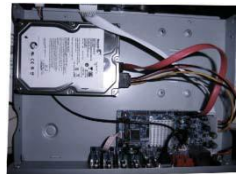
③ connect hard disk and mother board
