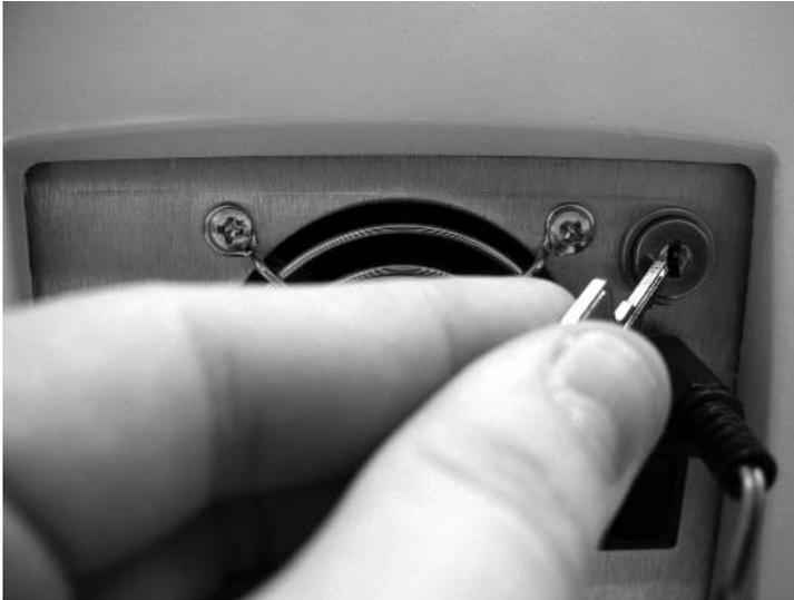
4. Remove the Safety Interlock Plug.
