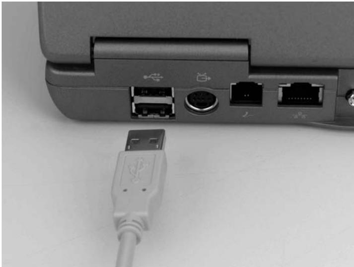
**NOTE:** The USB thermometer comes in two segments—a USB adapter, and the USB thermometer itself. First, connect the USB thermometer to the USB adapter. Then plug the USB adapter into the laptop.
