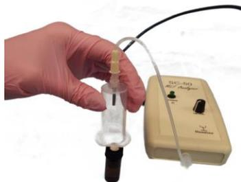
**Figure 7.** Position the opening of the vial insertion assembly over the vial.
