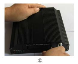
Make sure whether power switch is turned on or turned off, if it is turned on, please use the key, turn the indentation on the "turn off" position.
