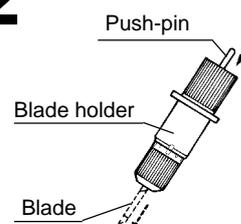
Press the push-pin and remove the blade from the blade holder.
