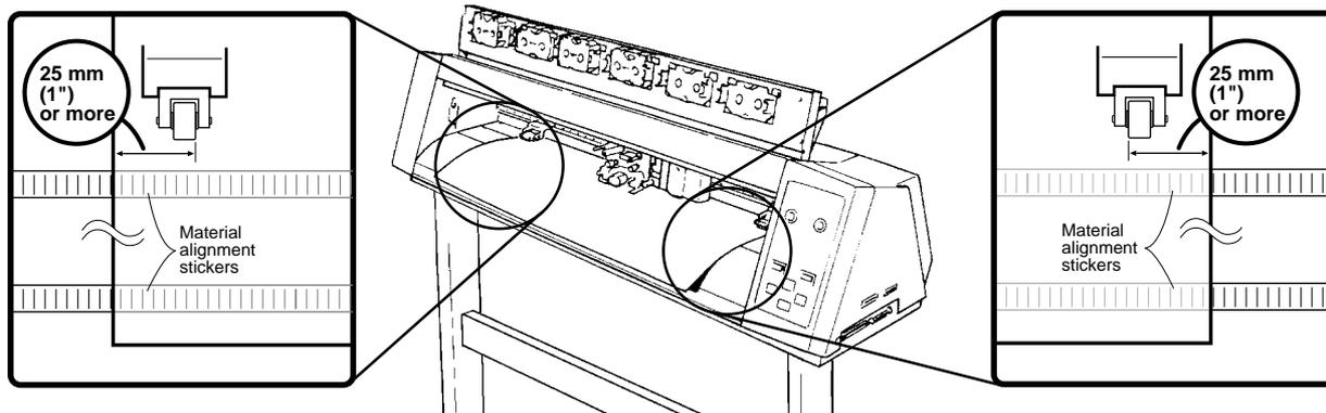
**4** Lower the sheet loading levers to secure the material in place.
