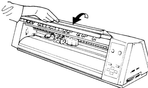
The FRONT COVER LED flashes if the front cover is not shut securely. Make sure the LED is lighted.
