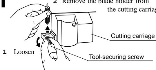
Leave the tool-securing screw loose. Tightening the screw makes it more difficult to install the blade holder.
