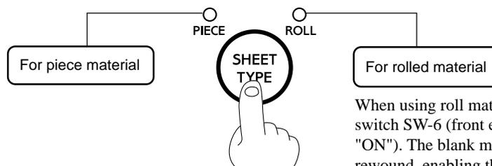
When using roll material, it is recommended that DIP switch SW-6 (front edge sensing) be enabled (set to "ON"). The blank margin toward the front of the unit is rewound, enabling the sheet to be used without waste.
