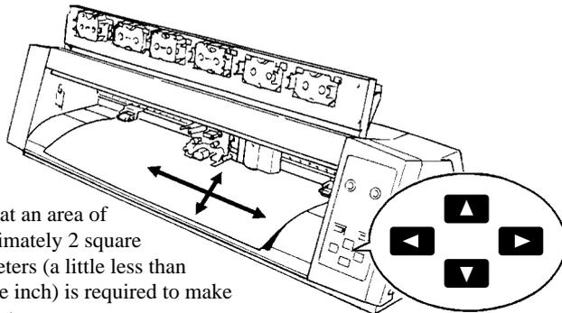
\* Note that an area of approximately 2 square centimeters (a little less than a square inch) is required to make a test cut.
