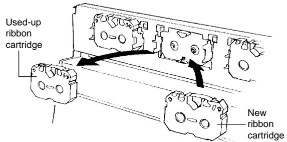
\* When a cartridge of a different color is installed, the COLOR LED flashes and printing is not resumed.
