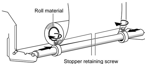
**6** Feed out the length of material to be printed or cut.
