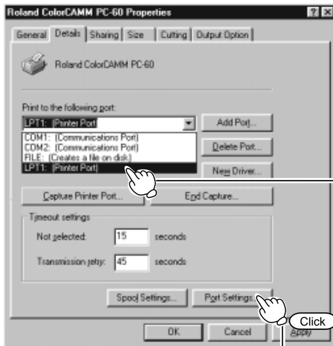
If a parallel connection is used for [Print to the following port:], select "LPT1: (Printer Port)".
