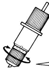
\* One full rotation moves the blade 0.5 mm up or down. (Scale shows gradations of 0.1 mm)
