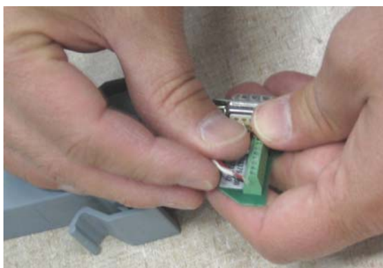
Figure 11-3 Connect Check Tag Wires
