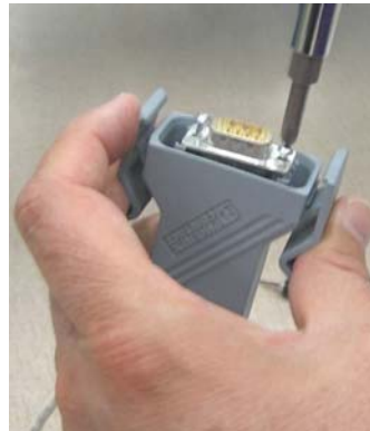
Figure 11-5 Securing Terminal Strip into Connector Housing
