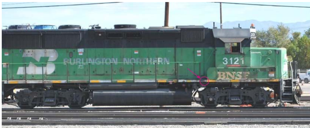
Figure 3-5 Right Front Placement of Tag on Locomotive
