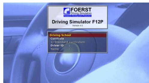
The menu is structured line by line and shows a cursor in the form of a red bar. In general, the button “Line” moves the cursor, while the button “Mode” activates or modifies a menu text.
