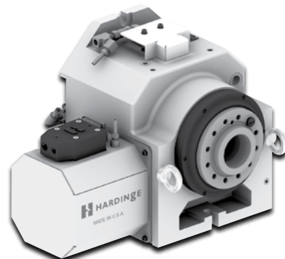
Reposition eyehooks to the face for lifting and mounting the Rotary Table Indexer on its back. Remove eyehooks before operating the unit.
