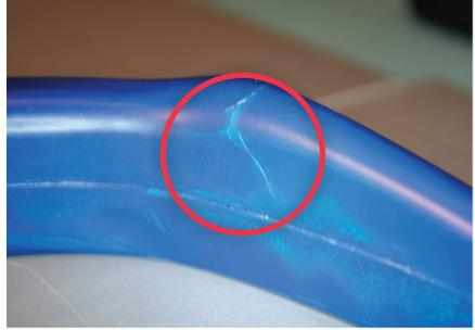
Camera Window Cracking
