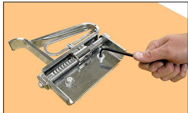
Figure 8 - Removing the SHCS
