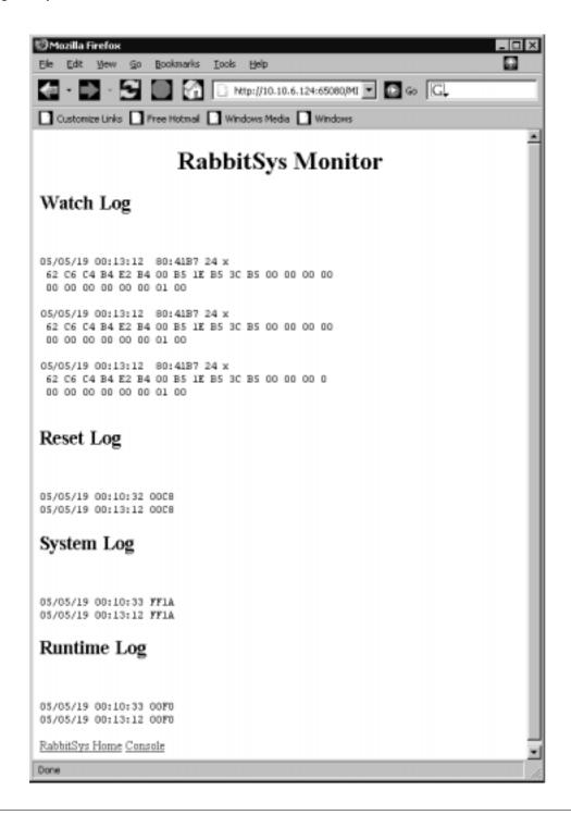
The monitor is accessible via both the console and HTTP. There are five types of monitor logs: watch, reset, run time, system and fatal (not shown). Monitor logs provides information on the state of a running or crashed program such as time, address, data, and cause.
