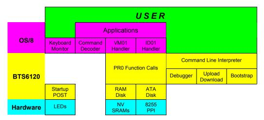
Figure 6 - SBC6120 Software Architecture
