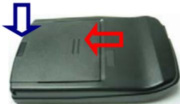
2. Pull out the battery cover. Insert battery in the unit
