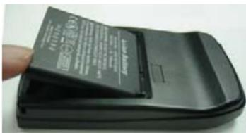
3. Put battery cover on to the cabinet. Then push down and force it forward to fit firmly
