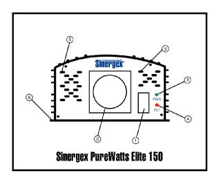
Power ON/OFF Switch. This switch turns the inverter ON or OFF for operation. When in the ON position the inverter will deliver power to the AC outlet.
