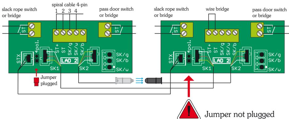
Note 1: When the jumper is used in the connection box, the slack rope switches/pass door switches are bridged in the main connection box. These contacts are then out of function despite the connected switches.
