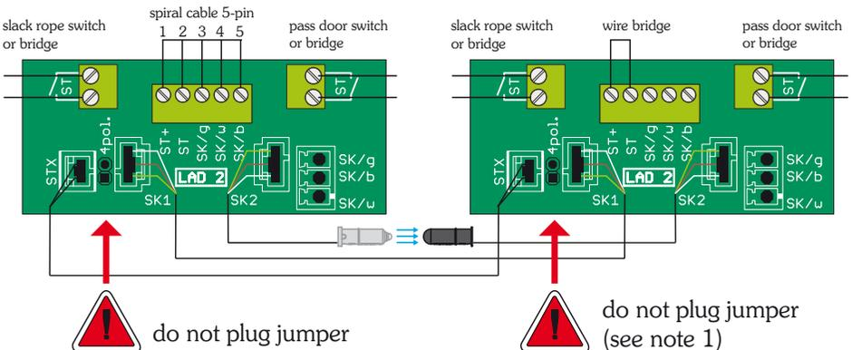
Note 2: If a jumper is used in connection with a 5-pin helix cable, the control is at risk of a short circuit. Use only with a 4-pin helix cable.
