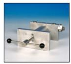
This system consists of an APC calibrator with a hydraulic, high pressure screw pump. System D is an easy-to-use calibration system. Place the pump on a flat surface and turn the handle to generate pressure. The calibrator may be adjusted to give the best viewing angle. The system includes a manifold for connection of the test device, a fine adjustment vernier valve (optional), and a reservoir for extra oil or water (optional).
