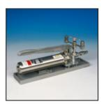
System F is an easy-to-use calibration system. The hydraulic pump makes it very easy to prime the system. The pump contains 75 in 3 / 1.23 I of liquid.
