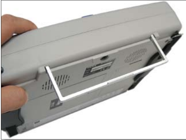
Pull-out steering wheel clip for tests performed inside the vehicle.
