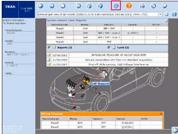
By selecting a vehicle and using the bulletin icon; a list of technical bulletins or test cards are accessible.
