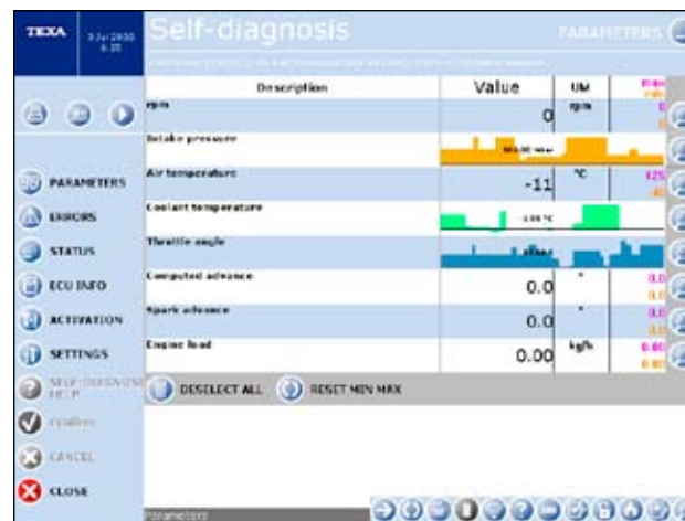
For example, by selecting the auto diagnostics program and connecting to the ECU, the list of engineering parameters can be accessed, and displayed on a graph.
