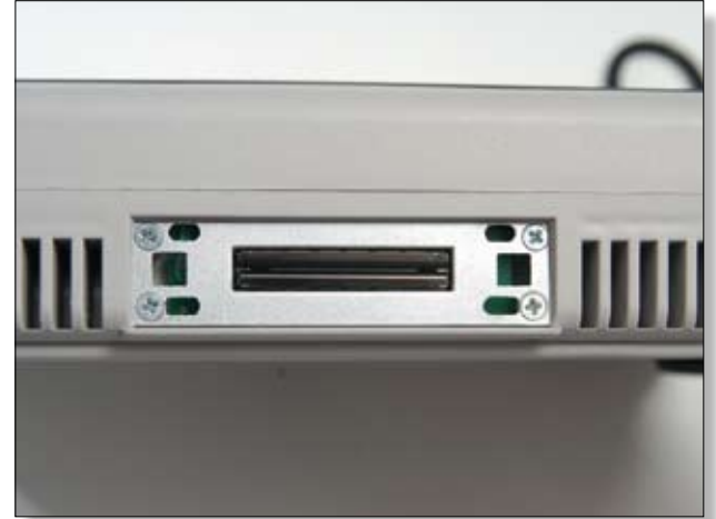
84-pin connector with dustproof tabs.
