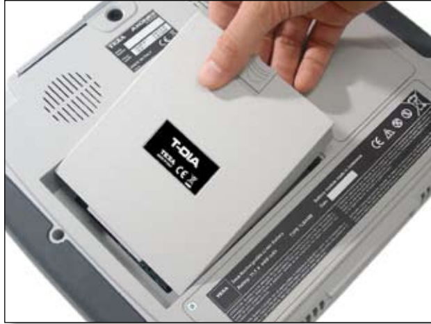
Module compartment. For fitting the specific working modules.
