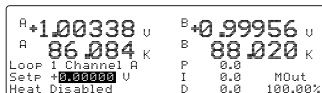
Normal Display with Temperature Setpoint Highlighted
