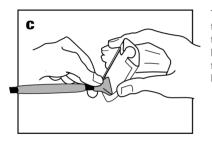
To close the lever, position the shoulder of the screw in the socket portion of the lever and align the tube with the clip at the front of the lever **(C)**.
