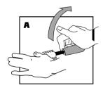
To open the lever, place the heel of your hand on the lower leech edge of the clamp and hook your middle fingers between the sail and the lever. Then pull back with your fingers prying the lever away from the leech, while pushing down the batten itself with your other hand **(A)**.
