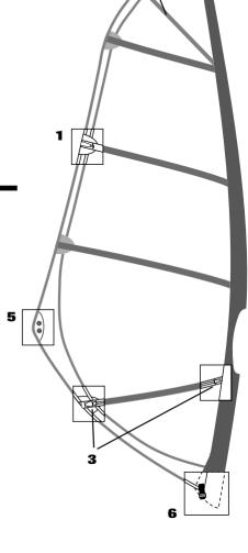
**Warning:** Do not over tension the battens. The screw should be extended only as much as necessary to remove wrinkles across the batten pockets. Over tensioning of the battens can damage the sail.
