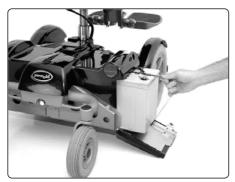
Loosening the first battery connection
