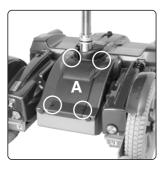
Remove the Center Chassis Cover (A)
