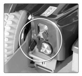
Wheel Lock Release Lever and Safety Catch
