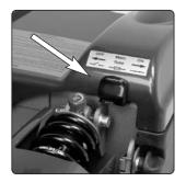
Lever for automatic Circuit Braker
